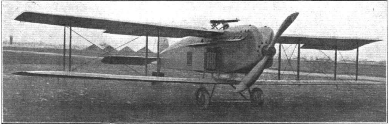
THE VICKERS F.B. 24 G.—The engine is a 275 h.p. Lorraine.
